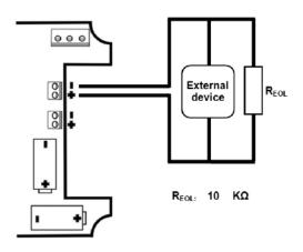
Wiring example for the relay switch output.
