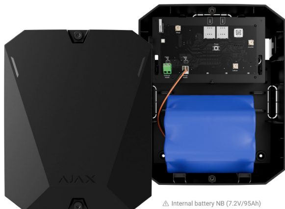
△ Internal battery NB (7.2V/95Ah)
