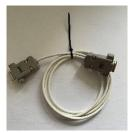
The loop cards for the Toccare Multi-loop require the below lead for upgrading the firmware.
