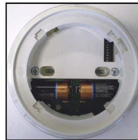
Picture 6 - primary and secondary batteries inserted
