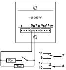
The 100-2037V input and output relay module combine in a single device supervised input and relay output characteristics.
