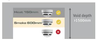
Voids deeper than 1500mm may be treated as a room when siting detectors below the ceiling - 150mm for heat and 600mm for smoke.
