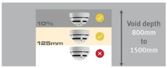
If the system category requires detection in any area, which has a void deeper than 800mm but less than 1500mm depth, detection should be provided in the void.
