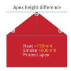
For ceilings that feature an apex: as long as the height difference between the apex and the height of the eaves is less than 150mm for Heat detectors or less than 600mm for Smoke detectors then these can be treated the same as flat ceilings.
